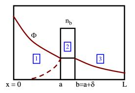
**FIGURE 1.** Geometry for 1D rf-blob interactions. The evanescent wave-field  $\Phi$  is launched from the left into a low density plasma region (1). It interacts with a blob of width  $\delta$  and density n<sub>b</sub> in region (2). Part of the wave is back-scattered (dashed), and the rest propagates through the blob and on into region (3).
