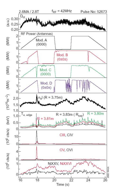
Fig. 2 Time history of  $D_{\alpha}$ , rf power, edge density, edge  $T_e$  and impurity spectral line intensities for the mixed-phasing shot #52673.
