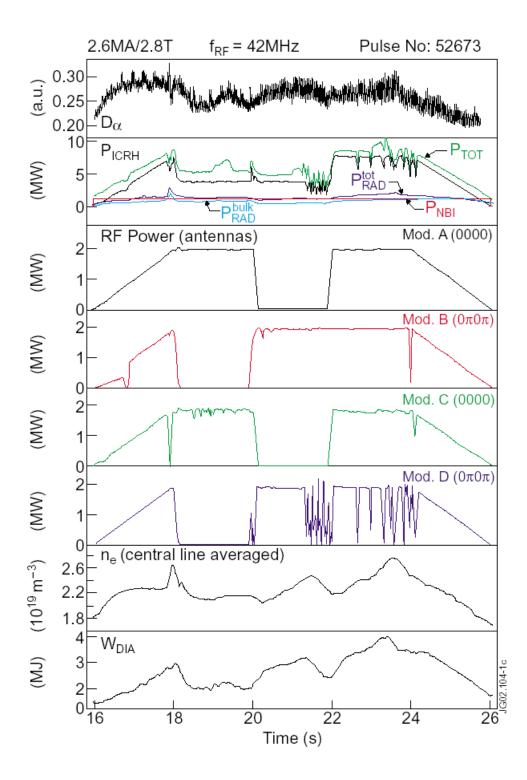
Fig. 1 Time history of  $D_{\alpha}$ , radiated power, rf power, line-averaged density and stored energy for the mixed-phasing shot #52673.
