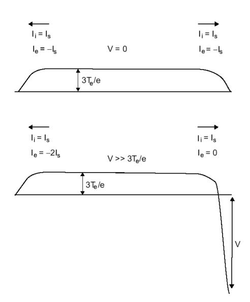
Fig. 5 Sketch of the dc plasma potential vs distance between the anode (left end) and cathode (right end) for the two capacitor plate sheath model. The cases eV = 0 and  $eV >> 3T_e$  are shown, where V is the applied potential difference between the plates. The arrows indicate the direction of current flow I<sub>i</sub> and I<sub>e</sub>, which is taken to be positive. Note that a net current flows to the cathode in the large-V case.
