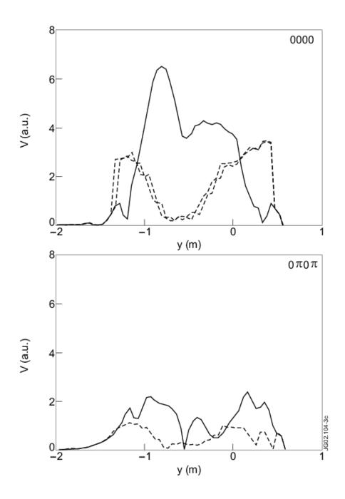
Fig. 3 Plot of poloidal sheath voltage distribution, V(y), with 0000 and  $0\pi0\pi$  phasings for three radial positions: one field line just in front (solid curve) and two just in back (dashed curves) of the FS tangency surface. Here, y is measured in meters from the symmetry plane (y = 0) and the units of V are arbitrary.
