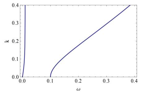
Fig. 7. Dispersion relation for the analytic wave model using the parameters of case (c) in terms of dimensionless parameters.
