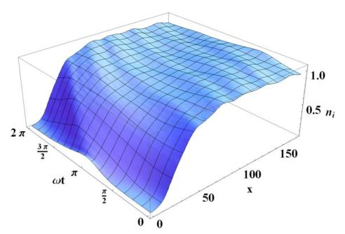
Fig. 3. Space-time plot of the ion density in dimensionless units for case (c):  $\Omega$ =0.1, b<sub>x</sub>=0.1,  $\omega$ =0.1, V<sub>pp</sub>=11.25. This more extreme limit of mobility and glancing angle exhibits a richer ion dynamics which includes the present of wave-like structures.
