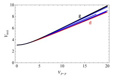
Fig. 6. Rectified voltage (including the thermal sheath contribution) for all the cases in Table I, superimposed. The highest curve is case (g), one of the most immobile, closely followed by case (e), both are shown in black. The lowest curve is case (d), the most mobile, shown in red.
