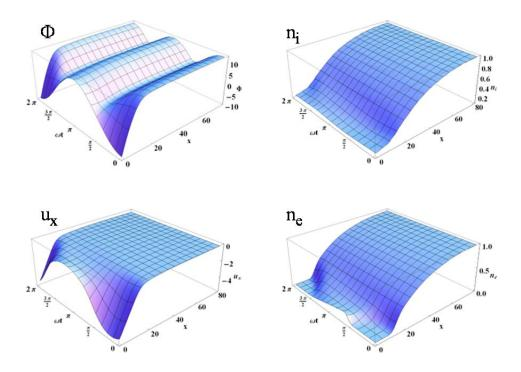
Fig. 1. Space-time plots of dimensionless rf-sheath quantities for case (a) of Table I:  $\Omega$ =0.1, b<sub>x</sub>=0.2,  $\omega$ =0.3, V<sub>pp</sub>=20 which is a marginally mobile, weakly magnetized glancing angle sheath. Shown clock-wise from upper left are the electrostatic potential, ion density, electron density and velocity normal to the wall. The wall, x = 0, is at the left and time (i.e. wave phase  $\omega$ t) advances in the direction receding to the left into the page.
