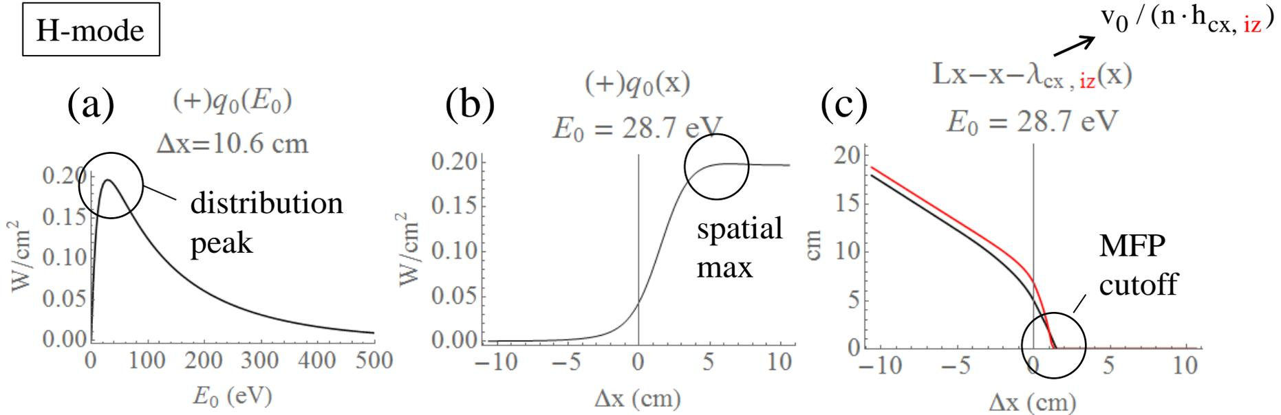
(a) The distribution function of neutral energy flux at the wall is maximized at  $E_0 = 28.7$  eV.
